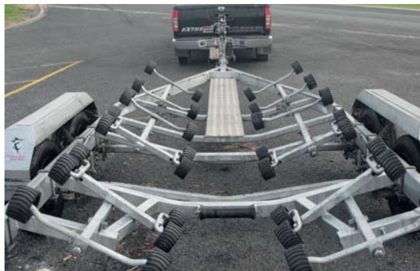
Twelve sets of multi-rollers support the boat well on the trailer while travelling, as well as making slipping it on and off a simpler task.
