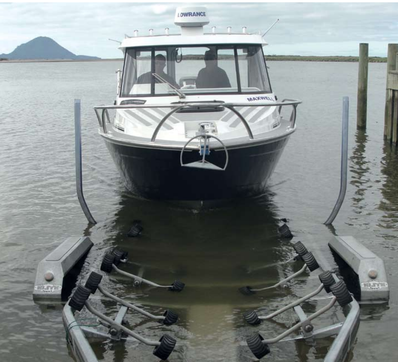
Guide poles and an extensive wobble-roller setup ensure the Extreme Game King 700 comes straight onto the trailer every time.
